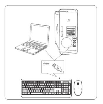
Insert USB plug of the mouse and keyboard into the USB port of your computer to work.
